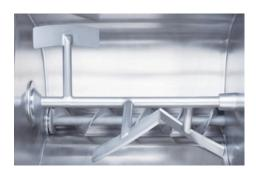
In grinding mode the mixing device supports the feeding process of the material into the worm housing. In mixing mode, the processing worm turns reverse in intervals to avoid that unmixed material can remain underneath it.
