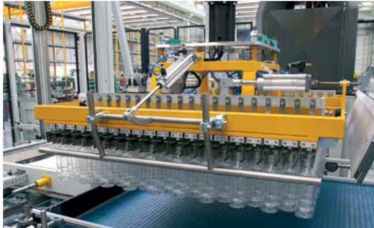
Side pressure gripping head for half depth crates
