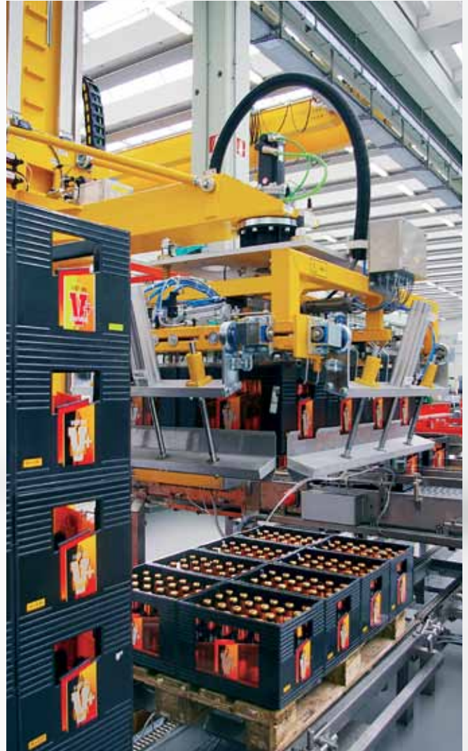
Transfer head with centering device and hooks for gripping crate layers at the sides
