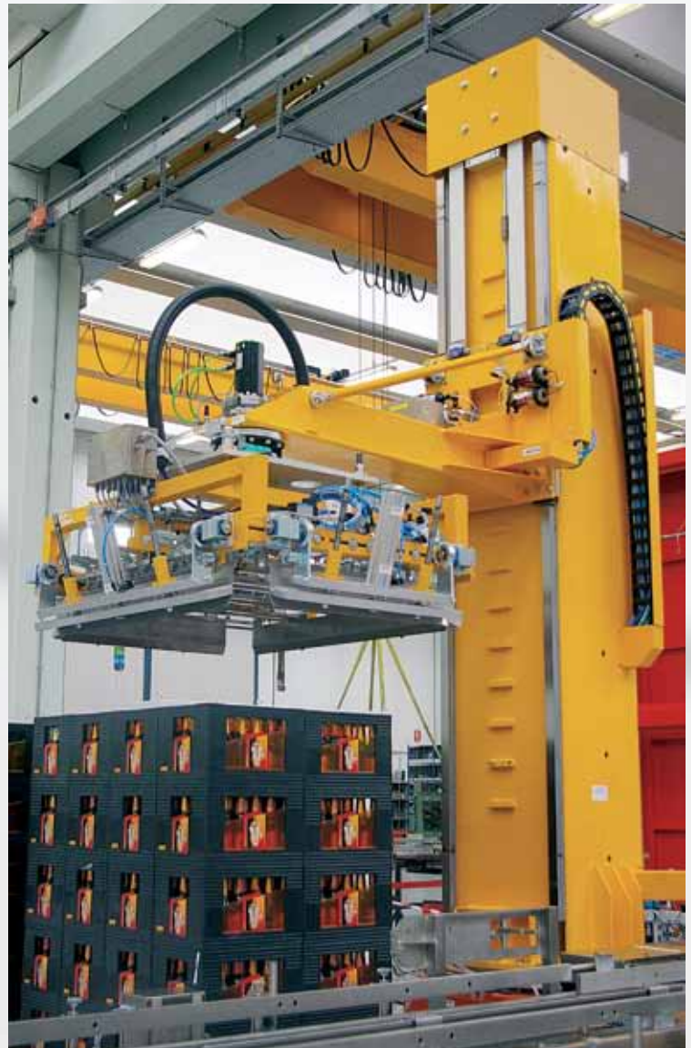
Single column main structure and lifting arm in painted steel
