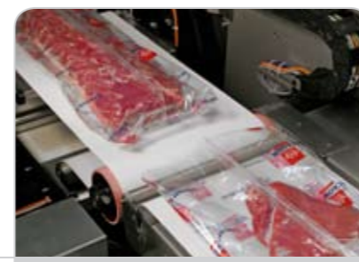
The product comes out of the machine inside the bag, ready for the vacuum process
