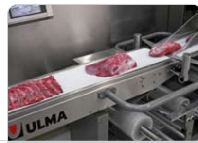
The system creates a bag and adapts to different product lengths without any changeover
