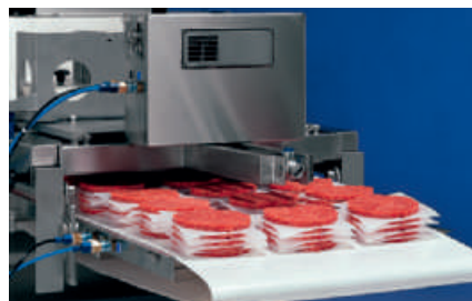
GEA Paper Interleaver to stack interlayered products automatically in a variety of arrangements
