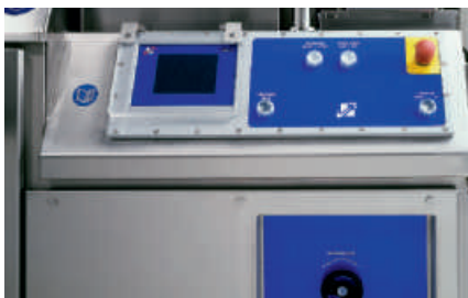
PLC control to set-up the optimum forming cycle and therefore secure the best product quality
