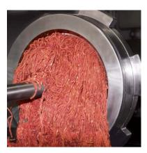
The PrimeGrind<sup>®</sup> 117 can grind up to 36,000 pounds (16,330 kg) per hour.
