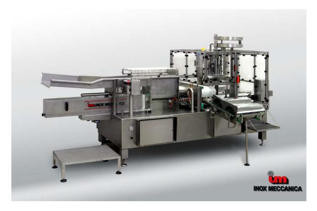
This model was designed to package proscutti, using stocking-net, at an elevated speed completely automatically.
