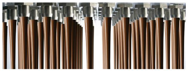
The SE 13-O Chain is a stationary mounted depositor. It has dynamic hopper movement and an offline feature for easy cleaning and to easily change depositing parts. Equipped with a built-in lifting table and integrated mold shaking.
