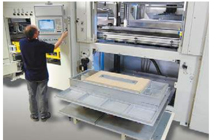
The conversion program supports the operator and enables automatic tool change in all stations.
