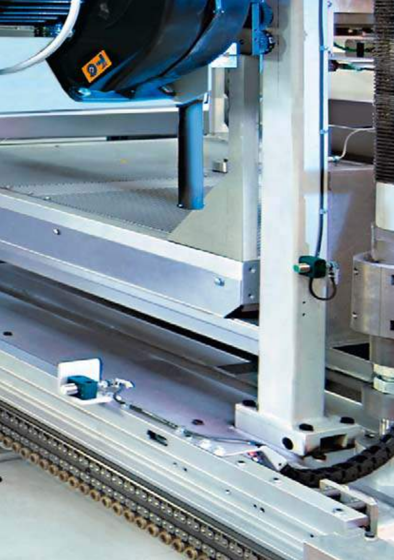
Sheet forming machine UA 155g with sheet loading device BE 155g equipped to work from roll stock
