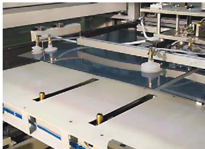
Centering of sheets on centering table
