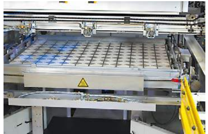
Higher output potential by application of pre-heating and off-station technology in the sheet loading device
