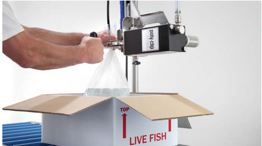
After filling with oxygen, the gate is closed and the clip is thus triggered.
