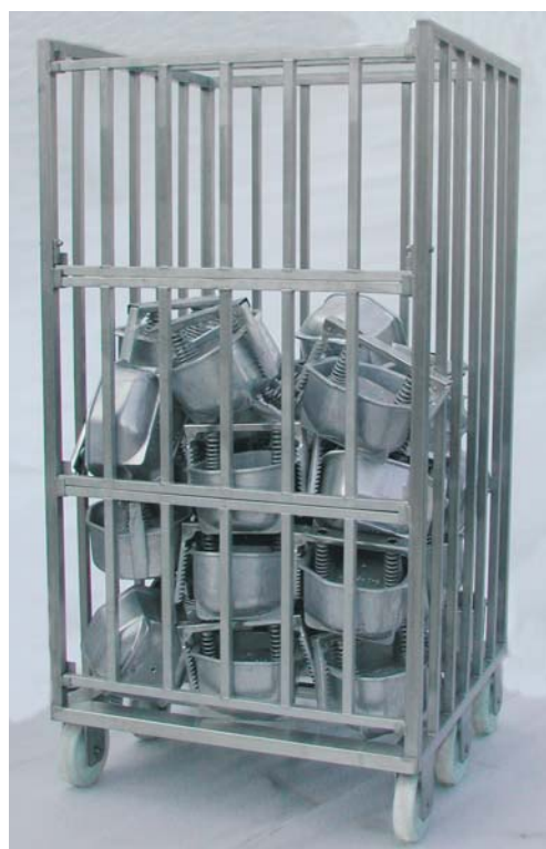
Loading trolley for ham forms
