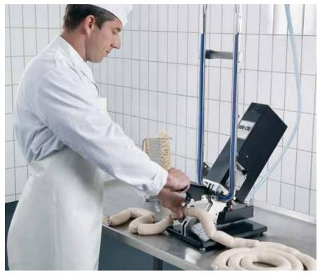
The DCD 600 securely closes all sheep, pork and beef rounds as well as synthetic casings up to calibre 60 mm
