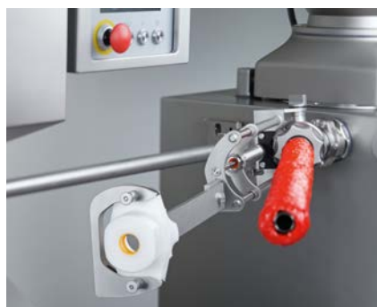
Brake assistant for fastest reloading of casings
