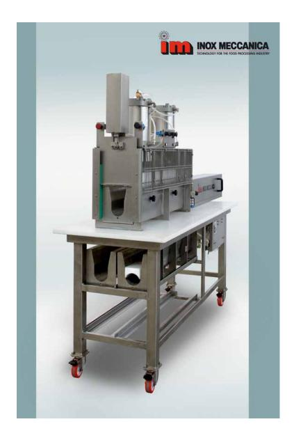
The machine has been built to resolve the problem of forming and calibrating salumis after the curing (neck- and belly-bacon rolls, salami, etc.) before they are sliced. The machine consists basically in a pressing-forming unit and an expulsion cylinder. The loading of the raw material and the expulsion of the formed product is effected through a loading door situated laterally on the mould.
