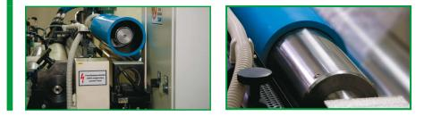
The laminating cylinder is an in-built air-cylinder onto which rubber sleeves can be pulled on from the side of the machine with the help of special valves. The rubber sleeve's width is less than the air-cylinder's width and equal to the laminating width.
