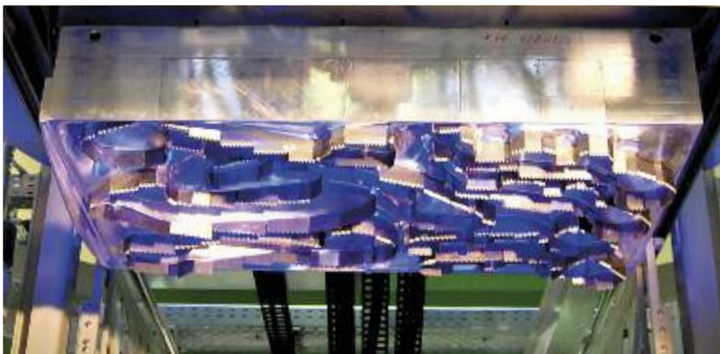
Upper part twinsheet Forming/Punching tool, Cutting knife moved out
