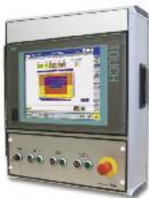
Operating panel UAR machines. Digitized function sequences enable field-proven operating philosophy of machine functions.
