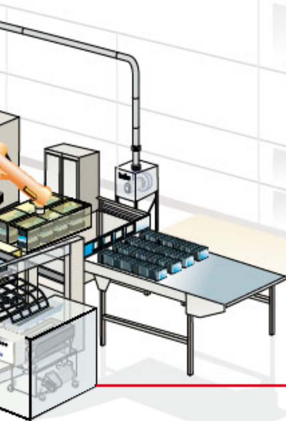
RDK 90 inline production line for forming/punching operation stacking with counting and transfer device
