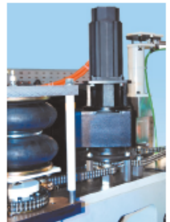
servo-driven height adjustment of upper table
