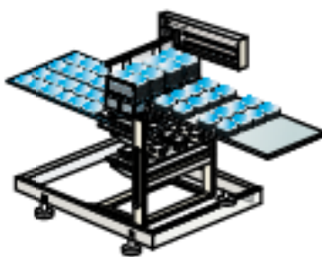
stacking device with counting and push-out device and stacking chute divided in two parts
