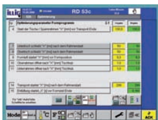
Screen page "optimization parameters forming program" The operating philosophy includes a structured operator guidance on the screen through the individual menu pages.
