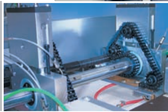
The pneumatic chain tensioning device continuously tensions the chain and thus ensures precise material transport
