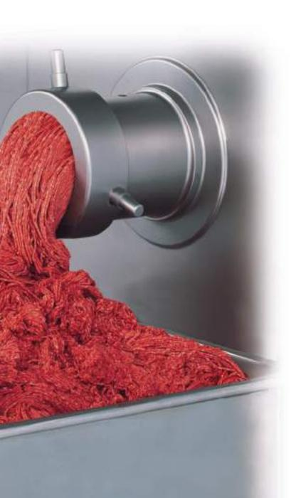
INDUSTRIAL GRINDER MEW 727 Size of cutting set 160 mm Capacity up to 4.500 kg/h
