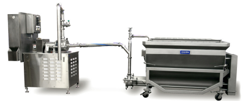
Horizontal Screw Loader feeding AR922MC system
