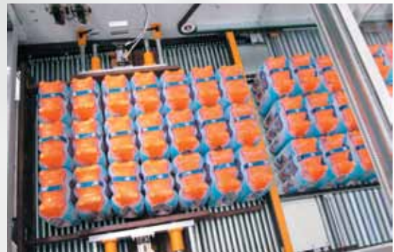
Layer compacting area
