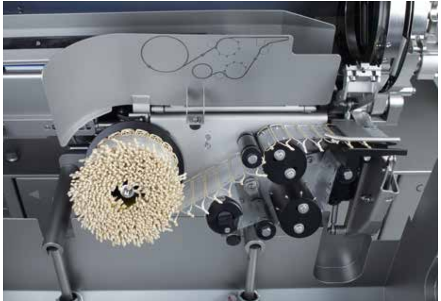
Reliable holding force for heavy products, e.g. in fibrous casing, cooked or matured while hanging on a loop.
