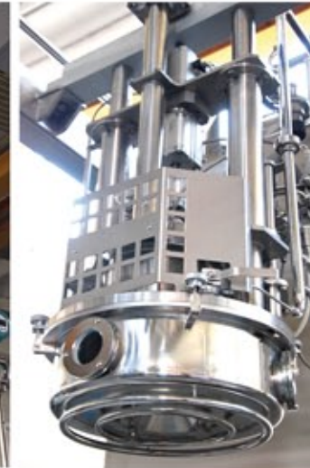
Detail of the filling head set up for 1 to 220 liters bags
