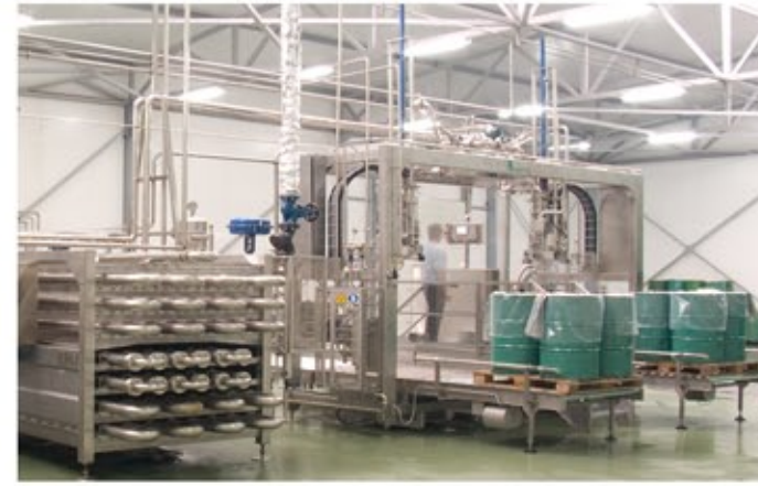
Filling machine mod. USA 152 provided with 220 liters bags in drums on pallet. Detail of the group complete with one "BOEMA" concentric pipes sterilizer
