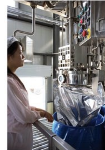
Filling phase of the 220 liters bag in drum
