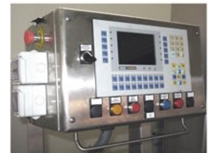
PLC for the management of the filling and running parameters' control phases and self-diagnosis system
