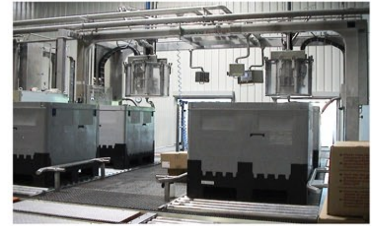
Filling machine mod. USA 152 provided with 1.200 liters "big-bag" type bags
