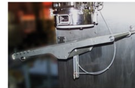
Device for 1 to 25 liters bags' filling, "bag in box" type
