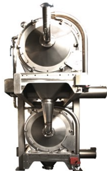
Front view of the group complete with screw conveyors for scraps' removal
