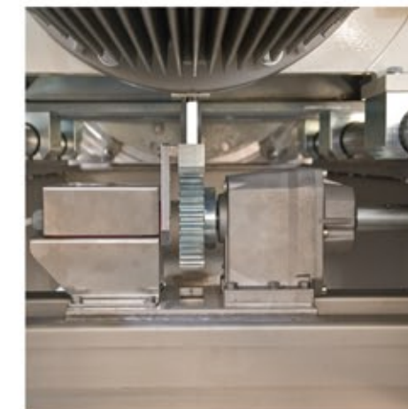
"Pinion-rack" transmission with manual powering by means of crank for rotor extraction from the machine body
