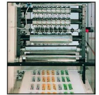
Twin vertical sealing rollers.
