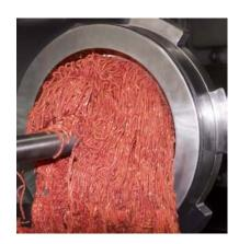
The PrimeGrind<sup>®</sup> CPG119-SF can grind up to 72,000 pounds (32,660 kg) per hour.
