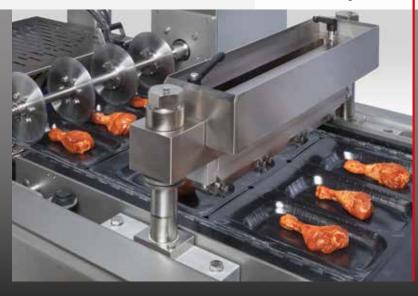
With a thermoformed skin pack, your product receives a skin-tight enclosure of a clear-transparent top film. This special skin film is being sealed onto the full surface of the bottom film without impairing the product. The result is a pack of excellent quality with enhanced food safety and the best possible product presentation – no matter if the product is presented hanging or lying at the point of sale.
