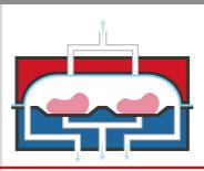
**1.** As soon as the sealing die has closed, the chamber is completely evacuated. The preheated top film is fed into the dome, heated further and plasticized.
