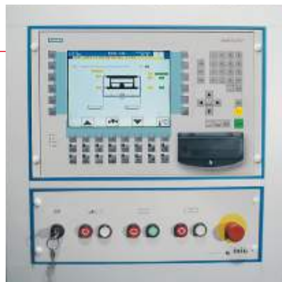
operating panel OP 37 and PLC unit
