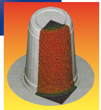
simulation – optimum wall thickness distribution
