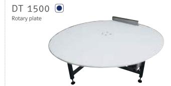
**External dimensions** Ø 1500 mm, 0.80 - 1.10 m\*\*\* Weight approx. 75 kg **Electrical connections** 1 phase, 230 V, 50 Hz/0.70 kW\*\*
