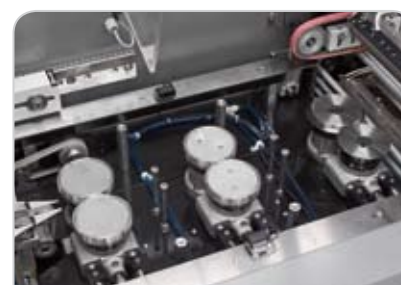
Longitudinal sealing system with tilting rollers
