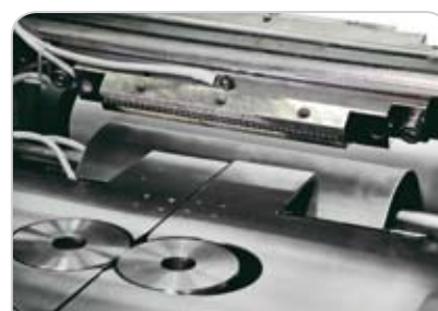
Cross cut sealing system with 2 jaws per shaft
