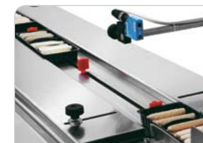
Photo cell control for "no-product no-bag" function
