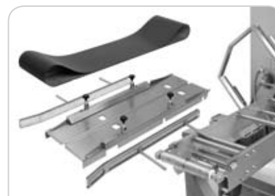
Tool-less detachable in-feed conveyor
