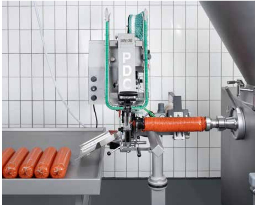
The PDC 700 closes all diameters up to 115 mm without any problems
