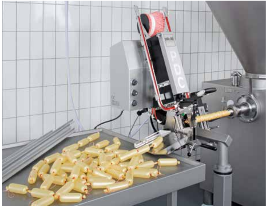
Products with diameters up to 90 mm can be produced quickly and safely with the PDC 600.
