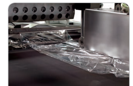
Continuous longitudinal welding system
