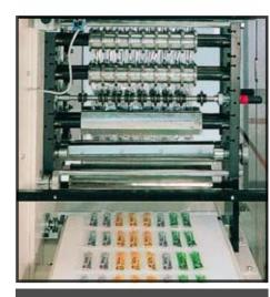
Twin vertical sealing rollers.
