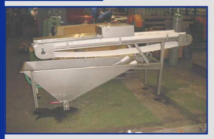
The washing belt conveyor is intended for use in fish processing by special herring and mackerel treatment lines. The washing belt conveyor as equipment connected to a slaughtering and filleting machine is provided for an additional washing of final products from the herring and mackerel treatment (fillet or carcass pieces) and their short-time interim buffering.
