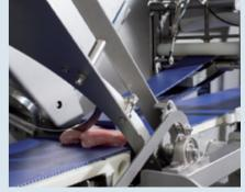
Changing the angle is fast and easy without the use of tools. The optimum gap between the infeed and outfeed belt is adjusted automatically (patent pending).
