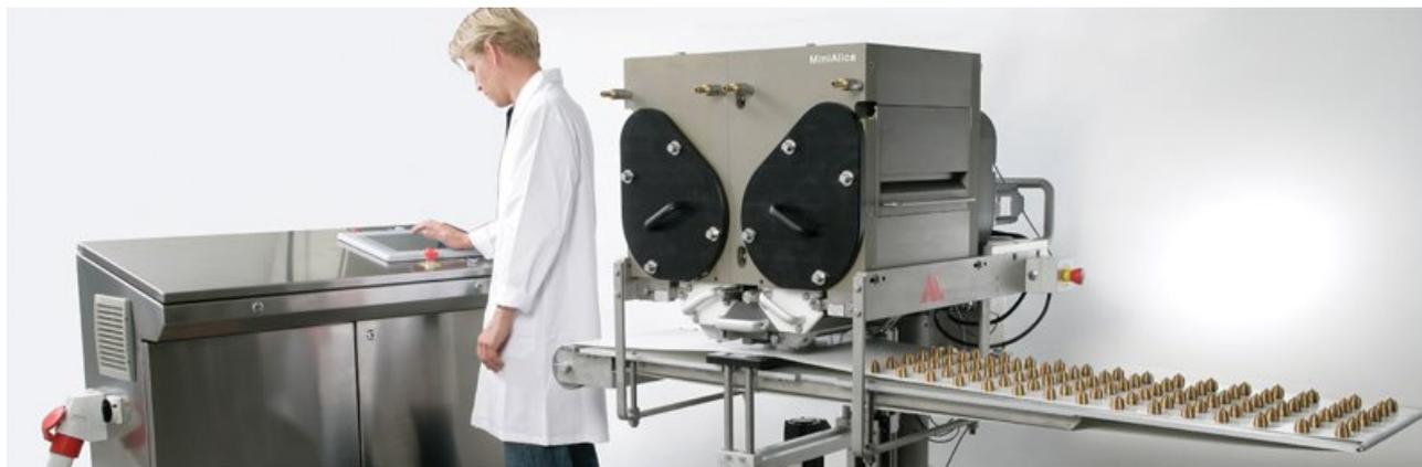
The Alice™ Single head configuration model provides flexibility for straightforward single extrusion and depositing
