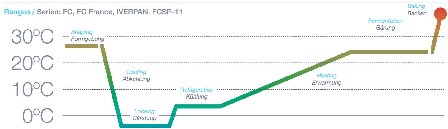
Controlled fermentation allows the professional artisan baker to rationalise production times. A drop in temperature to -1°C blocks all enzymatic activity. Correct moisture level and temperature parameters, along with the optimum design of the chambers, prevents any condensation in the product, leading to fresh, aromatic bread.
