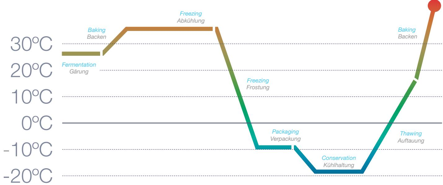
The recently baked pieces, still hot, are blasted at -18°C in the heart, thus maintaining all the properties of the product as if it were recently baked. Production is always distributed to sales points in line with the cold chain, which is key in this process.
