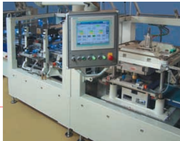
screen operating panel with sealing and punching unit
