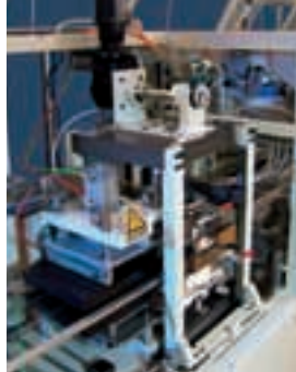
forming station with upper and lower tool part
