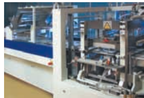
multiple gripper system and sealing station
