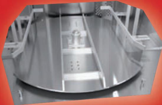
New ball coupling which facilitates coupling between the resting rack and the platform. A magnetic detector ensures correct functioning of the carriage stops. Optional universal platform.
