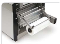
Pneumatic precision winding reel holder
