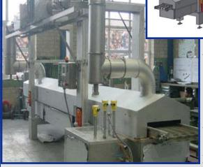
The B 400 / 4000 frying machine is designed for use in fish processing by special processing enterprises. The machine can be used as a single machine with operatively organized raw products supply and finished products discharge as well as by interlinked production lines. The machine fries the fishes prepared by salting, flouring or bread-crumbing or fish parts, particularly cutlet pieces.
