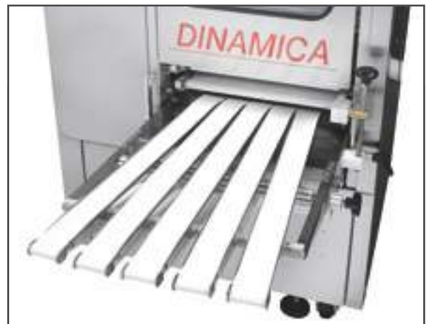
Finger belt to connect the Dinamica with a moulding station or a line (Optional).
