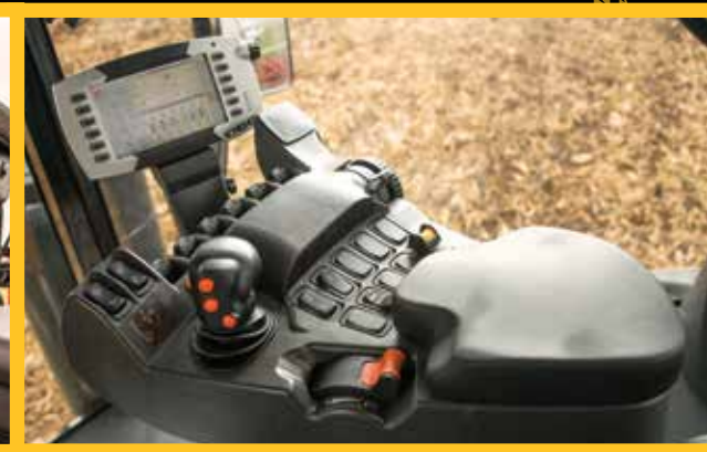
Industry-exclusive TMC (Tractor Management Center) armrest puts core functions at the operator's fingertips
