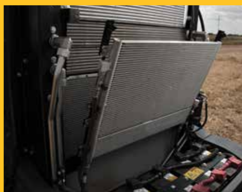
Engine cooling package with easy-to-clean two-plane design
