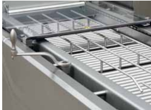
Employing a roller belt that is adjustable in height prevents heavy products from sagging.
