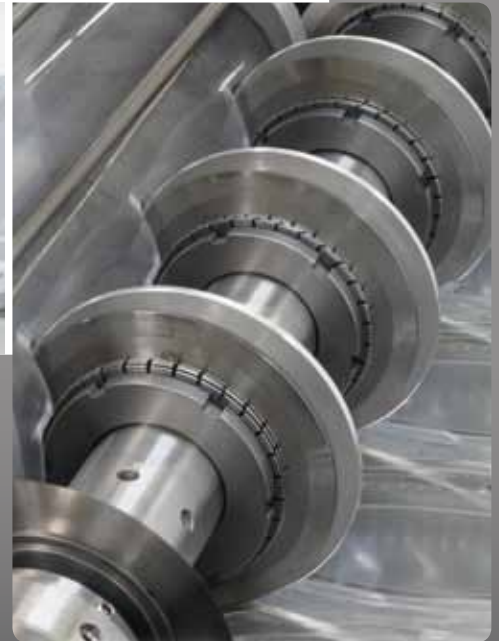
In order to prevent "cat nails", i.e. sharp-edged corners of the rigid film, apply the roll shear strip cutting in addition to the cross strip punch.
