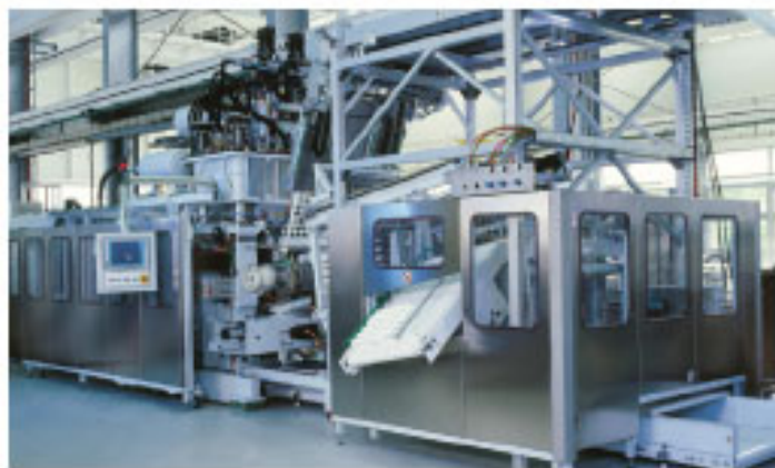
RDM 78 K automatic pressure former for forming/punching technology
