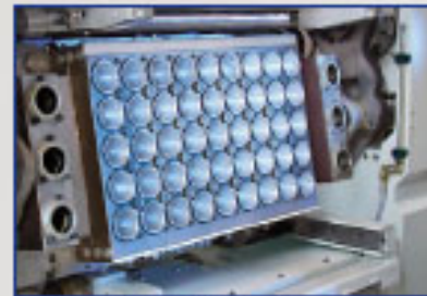
45-up forming/punching tool for RDM 78 K
