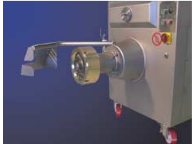
Optional: 66 Size Head and Safety Interlocked Discharge Guard fitted to a Stainless Steel Barrel, Feedscrew and Aluminium Bronze Lock Ring.
