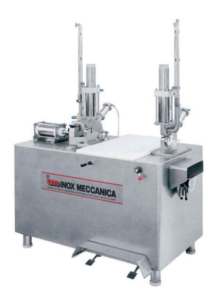
This machine has been designed to carry out the sealing of encased products through the use of aluminium clips.
