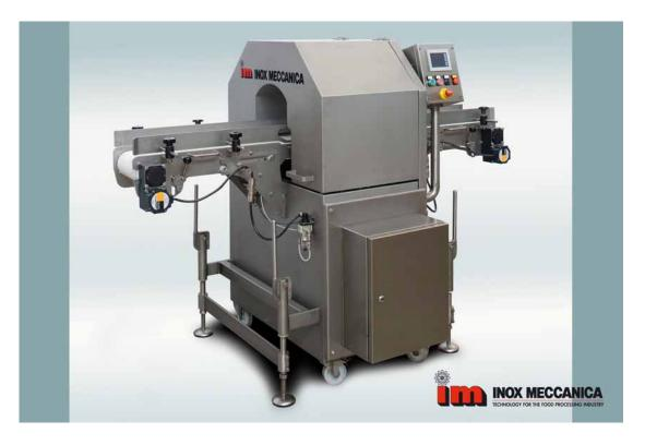
Automatic machine for tying in continuous, available in two distinct versions: model "S" for tying salumis already filled in casing like neck-bacon, belly-bacon, etc. and the model "R" for products consisting in one or more pieces rolled together or overlapped like roasts,
