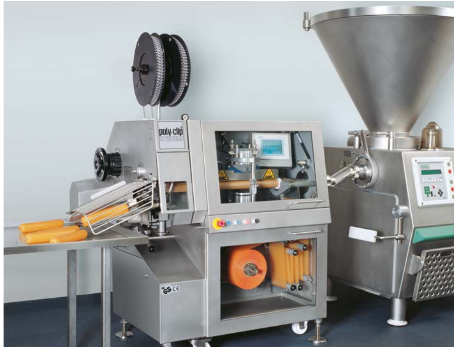
Efficient packaging of explosives using the TSCA 65 D
