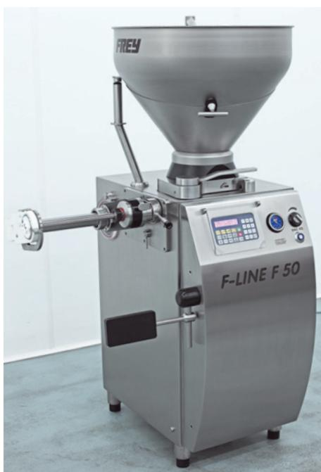
The standard F-LINE F50 model is equipped with a divisible **90 litres filling hopper**. The charging of the hopper as well as the intermediate cleaning is made easier.
